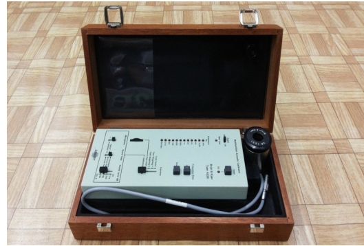
Gambar 2. Multi frequency sound calibrator (MFSC)
