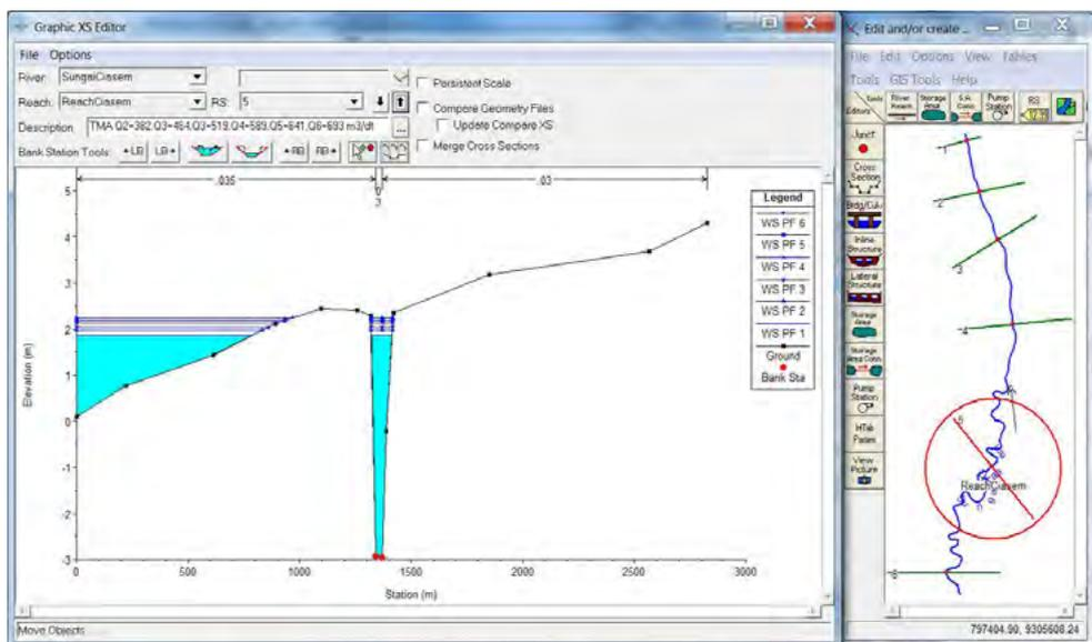
Figure 4. Inundation height on each cross section for the maximum flood-plan discharge in the periods of 2, 5, 10, 25, 50, and 100 year in river station (RS) 5
