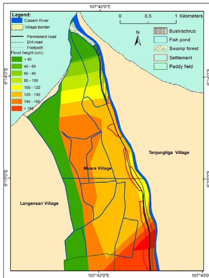
Figure 5. Inundation height caused by river flood
