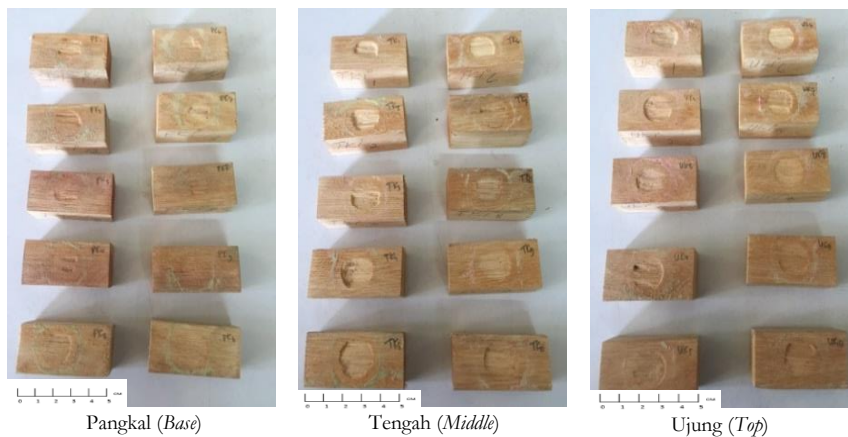
Gambar 5. Serangan rayap kayu kering pada kayu balam (teknik infus) Figure 5. Dry-wood termite attack on balam wood (infusion)
